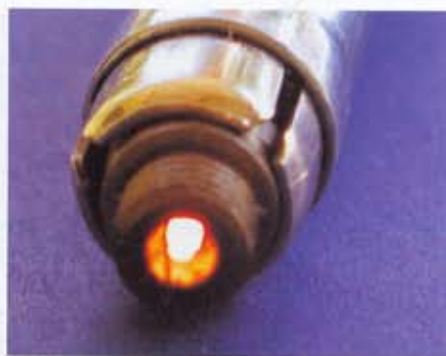
Glo plugs don't cost much and they do wear out. If the element loses the shine, gets pitted, frosty, badly distorted or only a few coils glow, chuck it away.
