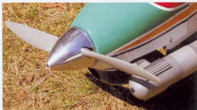
The simplest way to get a reliable idle on an inverted engine is raise the nitro content of the fuel.
