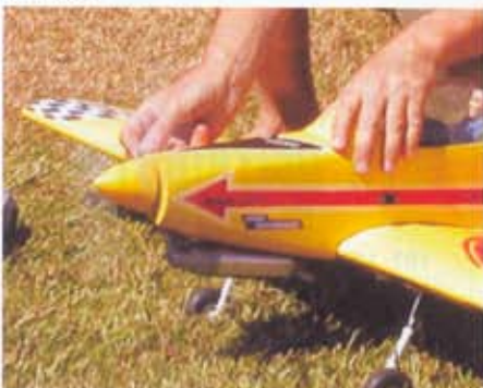
Tuning the needle valve for max rpm on the ground will give a lean run and cause overheating.
