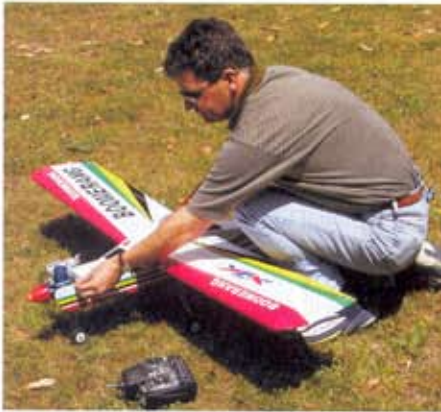
Always adjust the mixture from behind the model. Never reach around the prop from the front.
