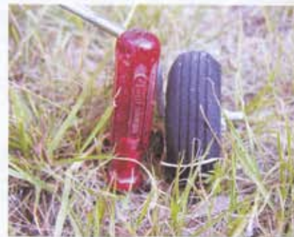
A safe and easy restraining system with one for each wheel.
