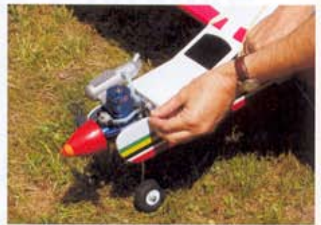
The rear needle valve was major safety innovation introduced by OS engines. Tuning on the left hand side keeps you away from the oily exhaust.
