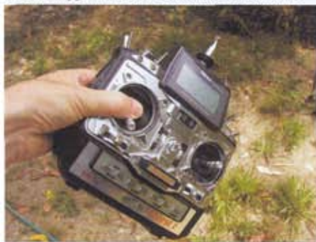
Prevent your fingers and even your plane flying away by starting the engine at a safe low throttle setting.
