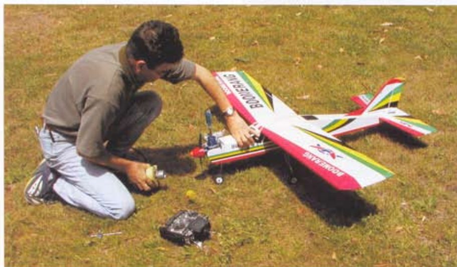
Keep your eyes out of line with the prop. Transmitter is within easy reach when you put the starter down. Aim the model away from other planes and people.
