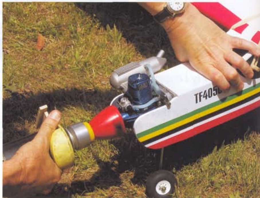
Line the starter up and push hard. When the engine is primed just connect the glo clip to crank it up safely for a perfect score. Fingers one prop zero
