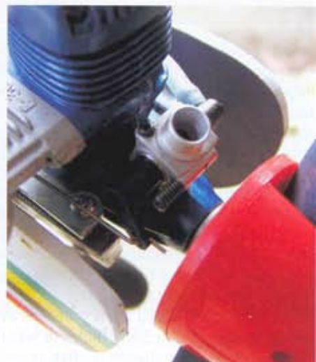
Metal to plastic is okay. The OS40LA no longer has a throttle stop. Back plate on the spinner helps reduce vibration.
