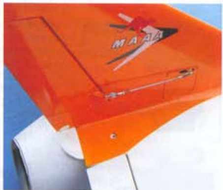
A short pushrod is recommended for high speed aircraft. This modern system is far superior to bellcranks, nyrods or cables.
