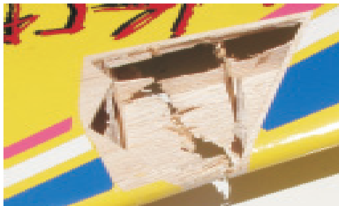
The damaged top of the Yak wing
