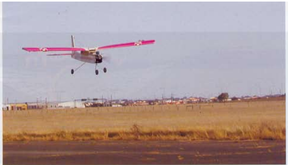
A slight correction to stay lined up, the right wing is level with the horizon. The model is ready to land so kill the power and hold the nose level.
