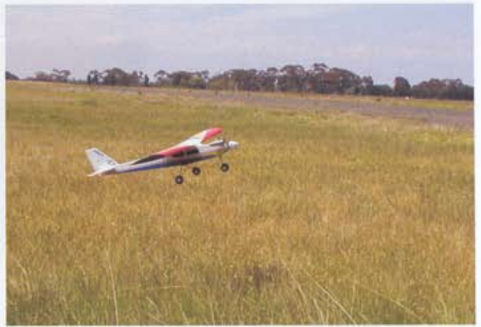
The nose is a bit high, just to emphasise the shot but unless you are really unlucky the model will be okay if you put it down slow.
