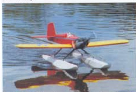
Original fibreglass undercarriage flexed too much without the support between the floats. A rotor blade off a 30 helicopter is an easy way to add an aerodynamic strut
