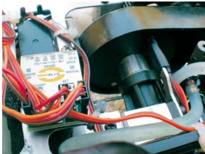
Installed ready to go the Revlock is set up for a standard six channel heli computer set.
