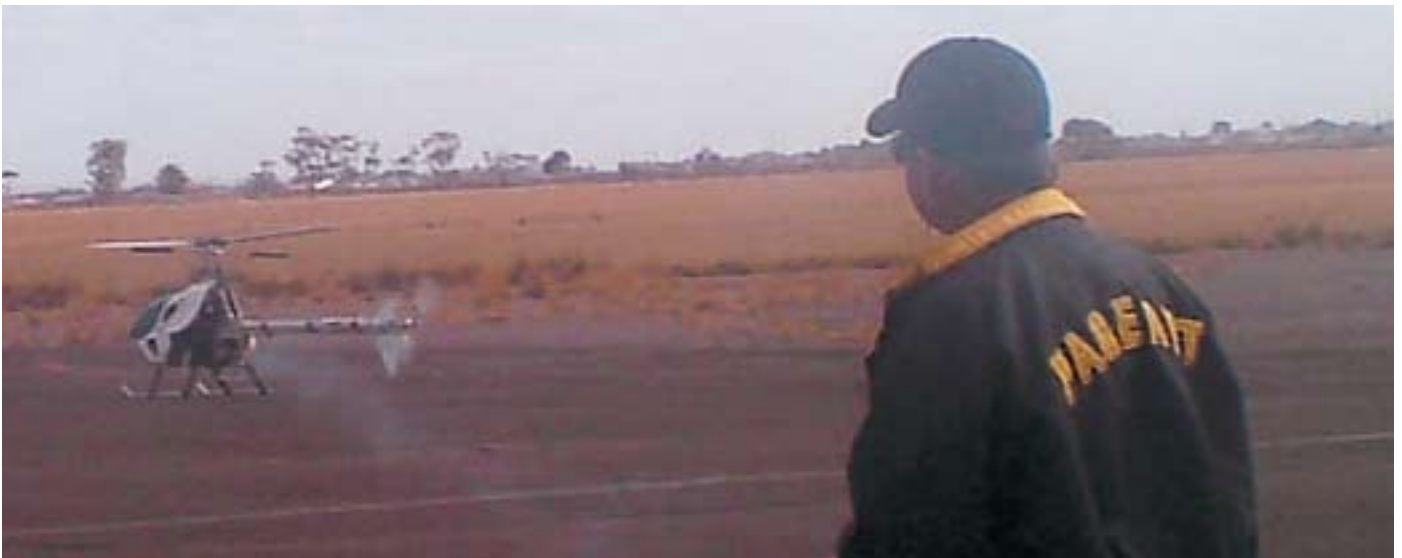
Lift off the machine off into wind. You can let it drift downwind to the right or apply right tail rotor and proceed slowly forward.
